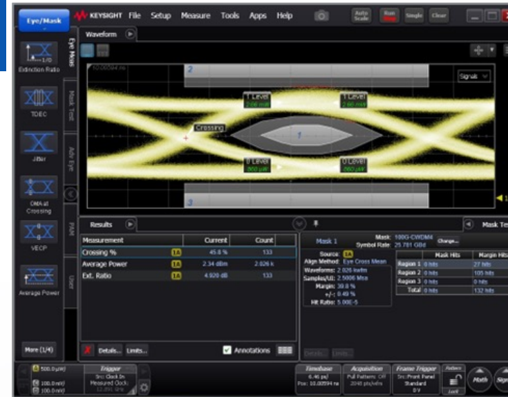
Tx & Rx Performance at 75C: ER = 4.92dB, EMM = 39.8%, Excellent BER
